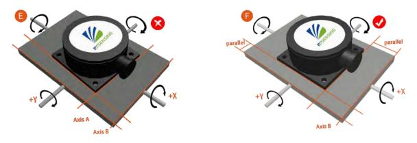
Finally, the mounting surface of the sensor and the surface to be measured must be fixed, the contact is flat, and the rotation is stable. The measurement error caused by acceleration and vibration should be avoided.
