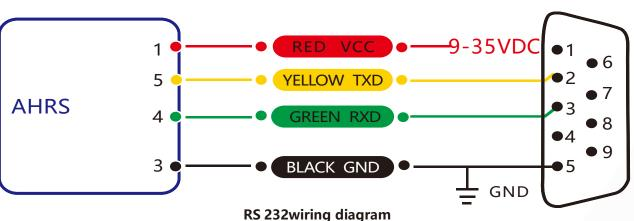
The RS232 interface needs to connect the ground wire of the product, the ground wire of the serial device, and the power ground.
