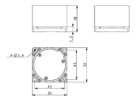
Note: Unfilled dimensional tolerances are performed in accordance with GB/T1804-2000 Class C.
