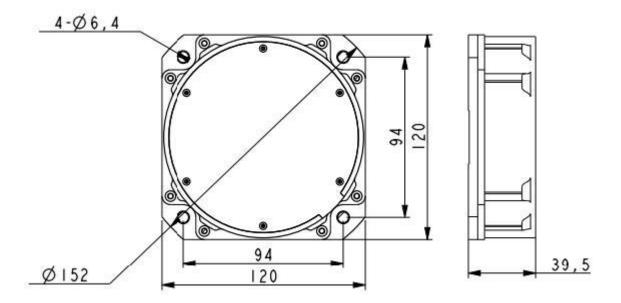
Note: Unfilled dimensional tolerances are performed in accordance with GB/T1804-2000 Class C.
