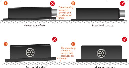
Secondly, the bottom edge of the sensor and the axis of the object to be measured cannot be generated at an angle as shown in Figure E. The bottom edge of the sensor should be kept parallel or orthogonal to the axis of rotation of the object to be measured. This product can be installed horizontally or vertically (vertical installation requires customization), and the correct installation method is shown in Figure F.
