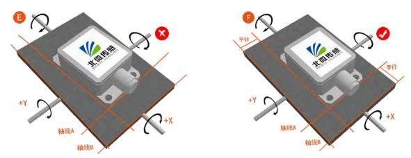
Finally, the mounting surface of the sensor and the surface to be measured must be fixed, the contact is flat, and the rotation is stable. The measurement error caused by acceleration and vibration should be avoided.
