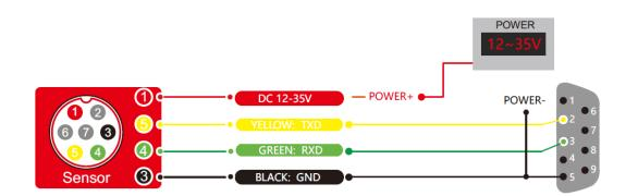
**EXERNSING** BWN420 Voltage Output Dual Axis Inclinometer
