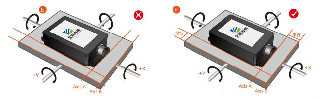
Finally, the installation surface of the sensor must be fixed with the measured surface tightly and smoothly, to avoid measurement error that may be caused by the acceleration and vibration.
