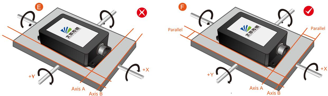
Finally, the installation surface of the sensor must be fixed with the measured surface tightly and smoothly, to avoid measurement error that may be caused by the acceleration and vibration.
