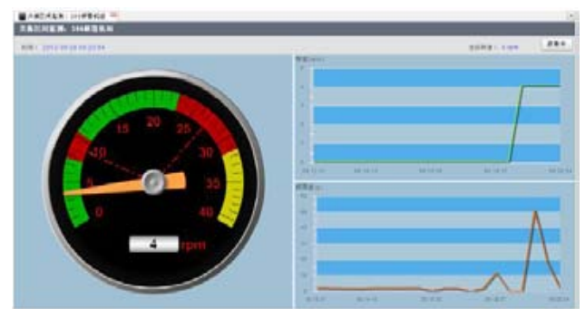
The overturning monitoring system of qingan wind power generator set
