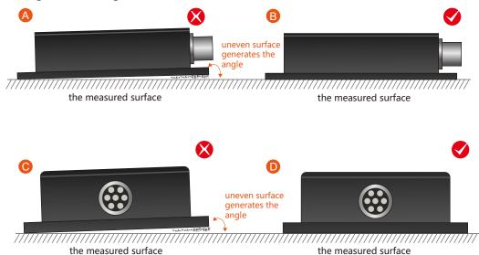
Secondly, the bottom line of the sensor and the axis of the measured object cannot have an angle as shown in Figure E. When installing, keep the bottom line of the sensor parallel or orthogonal to the axis of rotation of the measured object. This product can be installed horizontally or vertically (vertical installation needs to be customized), and the correct installation method is shown in Figure F.
