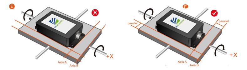
Finally, the mounting surface of the sensor and the surface to be measured must be tightly fixed, smooth in contact, and stable in rotation, and measurement errors due to acceleration and vibration must be avoided.
