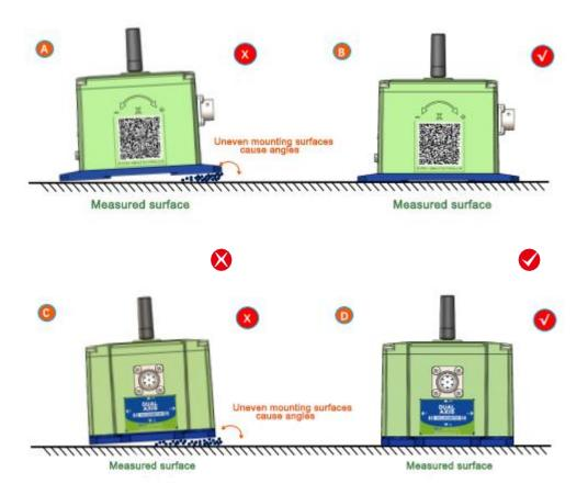
Secondly, the bottom line of the sensor and the axis of the measured object cannot have an angle as shown in Figure E, and the bottom line of the sensor should be kept parallel or orthogonal to the axis of rotation of the measured object during installation. This product can be installed horizontally or vertically (vertical installation needs to be customized), and the correct installation method is shown in Figure F.
